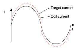
Coil current does not have optimum shape
