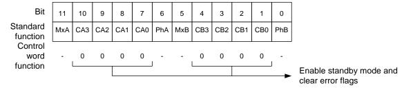
Programming current value "0000" for both coils at a time clears the overcurrent flags and switches the TMC236 into a low current standby mode with coils switched off.
