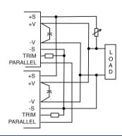
N+1 redundant connection adjustable output voltage
