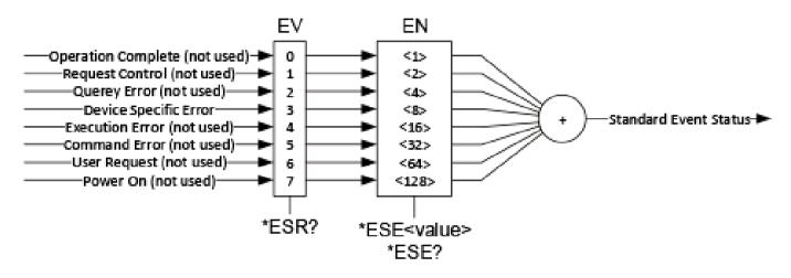
The Standard Event Status Register takes the standard SCPI structure. The eight individual condition inputs are:
