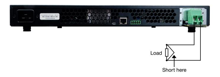
It is important that a good short with heavy wire is made as failure to do this will result in a poor remote sense calibration.
