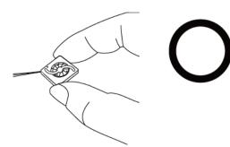
Don't pull fan with lead wires.
