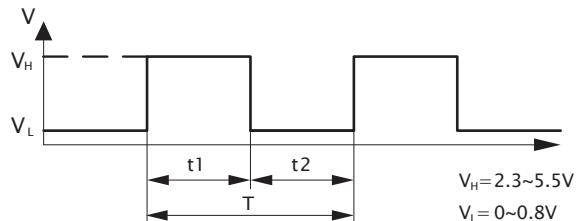
$$1. \text{ Period : } T = \frac{1}{f_{\text{PWM}}} = t_1 + t_2 (\text{sec})$$
