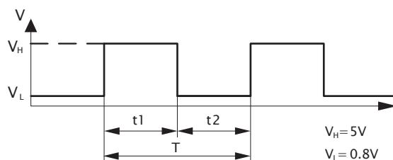
$$1. \text{ Period : } T = \frac{1}{f_{\text{PWM}}} = t_1 + t_2 (\text{sec})$$
