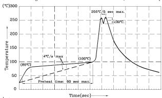
1.Recommend pre-heat temperature of 105°C or less (as measured with a thermocouple attached to the LED pins) prior to immersion in the solder wave with a maximum solder bath temperature of 260°C 2.Peak wave soldering temperature between 245°C ~ 255°C for 3 sec
