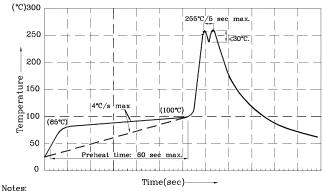
1.Recommend pre-heat temperature of 105°C or less (as measured with a thermocouple attached to the LED pins) prior to immersion in the solder wave with a maximum solder bath temperature of 260°C 2.Peak wave soldering temperature between 245°C ~ 255°C for 3 sec
