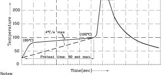
I.Recommend pre-heat temperature of 105°C or less (as measured with a thermocouple attached to the LED pins) prior to immersion in the solder wave with a maximum solder bath temperature of  $260^{\circ}$ C 2.Peak wave soldering temperature between  $245^{\circ}$ C ~  $255^{\circ}$ C for 3 sec
