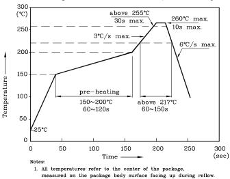
Reflow Soldering Profile for SMD Products (Pb-Free Components)
