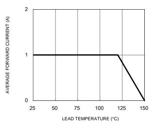
Fig.1 Forward Current Derating Curve
