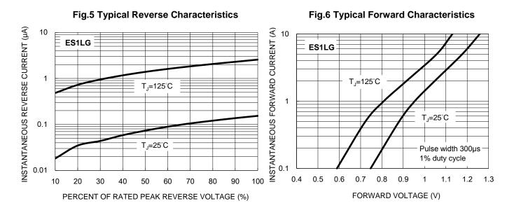
Fig.7 Typical Reverse Characteristics
