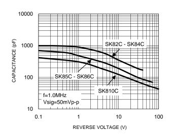
Fig.3 Typical Reverse Characteristics
