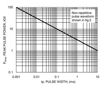
Fig.2 Pulse Derating Curve
