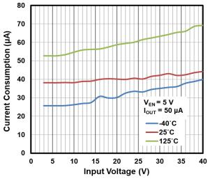
Figure 8. Current Consumption vs. Input Voltage
