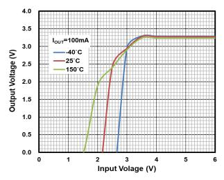
Figure 5. Output Voltage vs. Input Voltage
