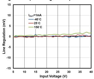
Figure 4. Line Regulation vs. Input Voltage
