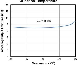
Figure 15. Watchdog Output Low Time vs.
