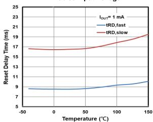
Figure 12. Power On Reset Delay Time vs.
