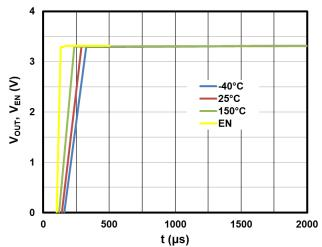
Figure 19. Output Voltage vs. time (EN switched ON)
