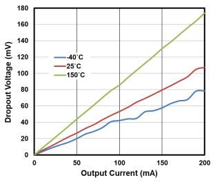
Figure 2. Dropout Voltage vs. Output Current
