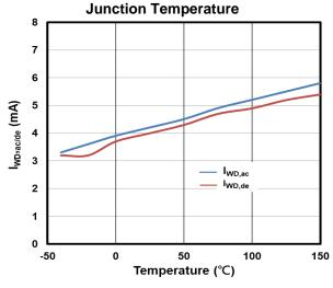
Figure 16. Watchdog Activation/Deactivation Current
