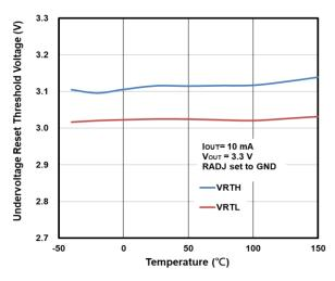
Figure 11. Undervoltage Reset Threshold vs.
