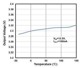
Figure 1. Output Voltage vs. Junction Temperature
