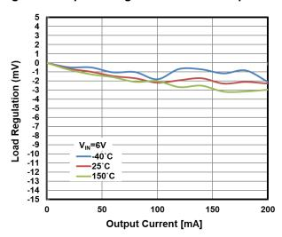
Figure 3. Load Regulation vs. Output Current
