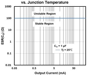
Figure 18. Output Capacitor Series Resistor ESR(C<sub>0</sub>) vs. Output Current
