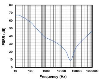
Figure 6. Ripple Rejection vs. Frequency
