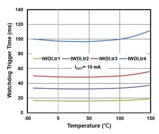
Figure 14. Watchdog Trigger Time 1,2,3,4 vs.
