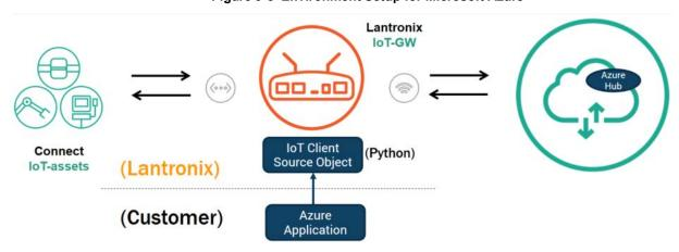
Python libraries are integrated into PremierWave 2050 software to support the Azure IoT SDK. This is represented above as "IoT Client Source Object." Your Azure application must be built on top of the PremierWave 2050 software. After connecting IoT devices to the PremierWave 2050, the PremierWave 2050 can then be connected to Azure Hub.
