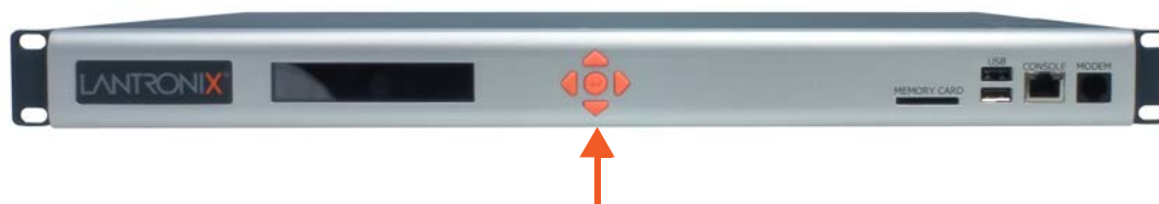
Figure 4-2 Front Panel LCD Display and Five Button Keypad (Enter, Up, Down, Left, Right)
