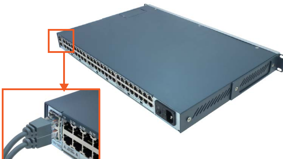
Figure 2-10 Dual Ethernet Network Connection
