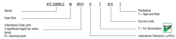
The above part number refers to a 506WLS Series, Case Size M, 0.47 µH inductor, K tolerance (±10%, typ.), with Tin Termination (T), 815 mA, tape and reel packaging..
