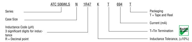
The above part number refers to a 506WLS Series, Case Size N, 1.47 µH inductor, K tolerance (±10%, typ.), with Tin Termination (T), 694 mA, tape and reel packaging..
