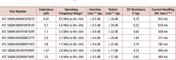
\*Lower -3 dB roll-off frequency \*\*Shunt Mounted \*\*\*Current for 100 °C temperature rise
