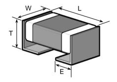
Stacked type CKG\*\*N : 2 chip capacitors.
