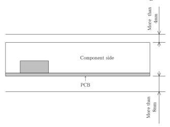
Keep 4mm space from the surfaces and sides of PCB. Especially, 8mm space is necessary from the solder surface.
