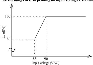
The following input voltage derating curve assumes maximum output power is 100%
