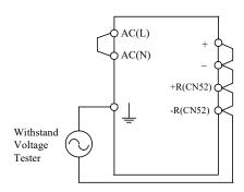
Note 1: This product have monolithic ceramic capacitor in secondary circuit to  $\frac{1}{2}$ . Some of the withstand voltage tester may generate high voltage at the matching with monolithic ceramic capacitor and may cause the unit damage. So, please check the waveform of applied voltage.
