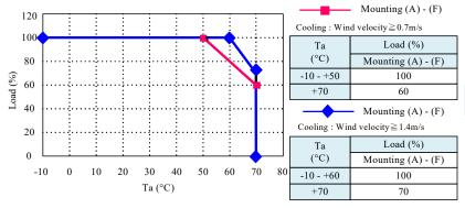
Electrolytic capacitor allowable Max temparature
