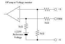
Fig.2-6 Internal TRM Circuit (For the Reference)
