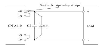
Fig.10-2 Remote Sensing is not used (Local Sensing)
