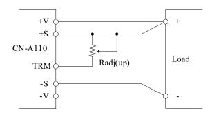
Fig.2-3 Connection for Output Voltage Trim Up
