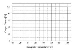
Fig.14-2 Derating Curve
