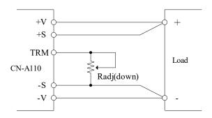
Fig.2-1 Connection for Output Voltage Trim Down
