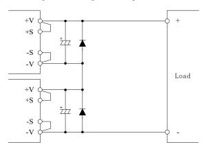
Fig.13-1 Series Operation due to High Output Voltage
