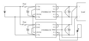
Fig.12-4 Variable Output Voltage (by Applied External Voltage)
