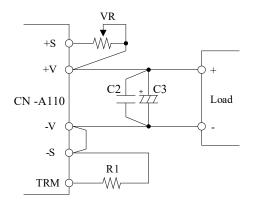
Fig.2-5 Example of Connecting External Resistor
