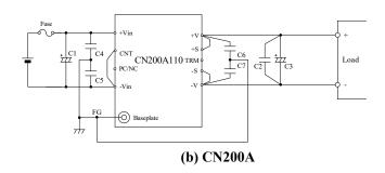
Fig.19-4 Example of connecting external application
