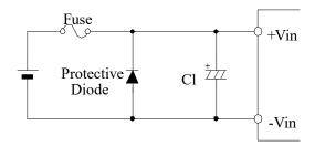
Fig.1-3 Protection for Reversed Connection of Input
