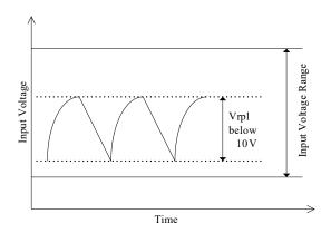
Fig.1-1 Input Ripple Voltage
