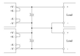
Fig.13-2 Series Operation due to ±Output
