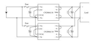
Fig.12-1 PC terminal Connection
