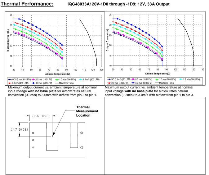
Thermal measurement location - top view
