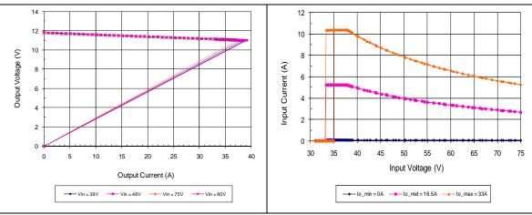
Output Current Limit Characteristics vs. Input Voltage
