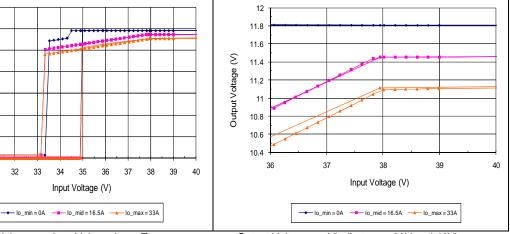
Typical Output Voltage vs. Low Voltage Input Turn-on and Turn-off at Ta=25C
