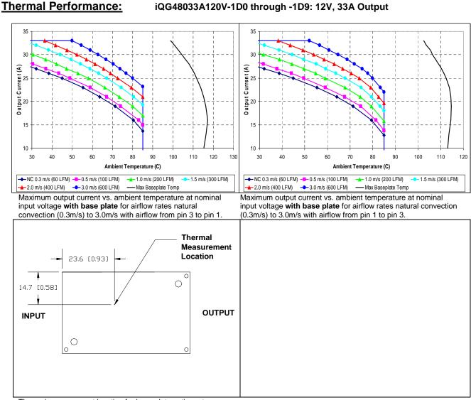
Thermal measurement location for base plate option – top view
