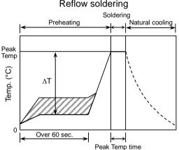
5-3. Recommended soldering peak temp and peak temp duration for Reflow soldering Pb free solder is recommended, but if Sn-37Pb must be used, refer to below.
