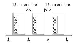
Provide punching, etc. to allow air to pass.
