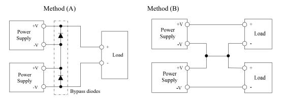
Note : In case of method (A), connect bypass diodes. If not, the unit might cause damage. Please select a bypass diode with maximum forward current rating more than output load current. And maximum reveres voltage must withstand each power supply output voltage.
