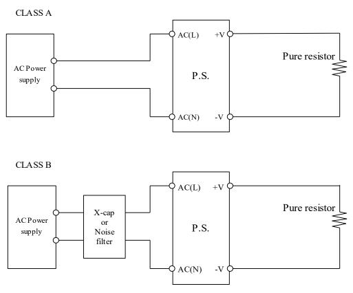
X-cap recommended : ECQU3A104MG(PANASONIC) or CTX104K310VP10 (CHENG TUNG). Noise filter recommended : RSEG-2001 (TDK-Lambda).
