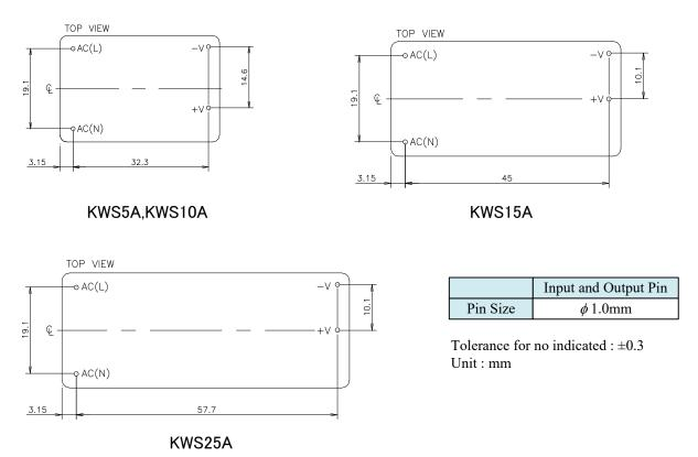
Fig.7-1 The mounting hole position
