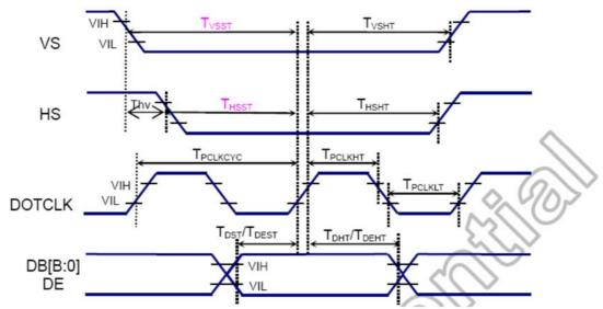
Figure 8.3: RGB interface characteristics
