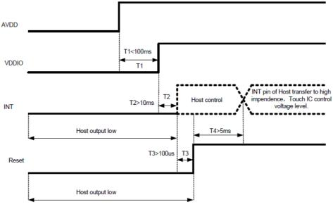
Fig.7 Power on diagram
