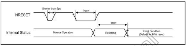
Figure 8.5: Reset input timing
