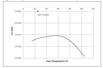
Figure 7: Typical DC ccy Shift vs. Case Temperature
