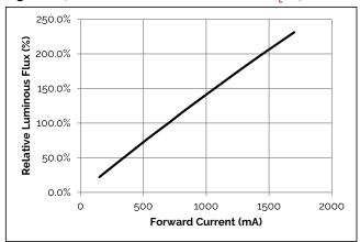
Figure 4: 590mm Relative Flux vs. Current, T<sub>c</sub>=25°C
