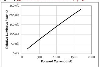
Figure 6: 1190mm Relative Flux vs. Current, T<sub>c</sub>=25°C
