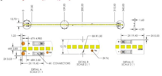
Figure 13: Drawing for BXEB-L0590U-xxx1500-C-C3
