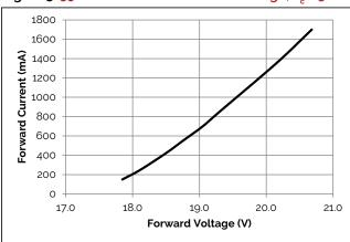
Figure 5: 1190mm Current vs. Forward Voltage, T\_=25°C
