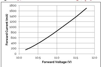
Figure 3: 590mm Current vs. Forward Voltage, T\_=25°C
