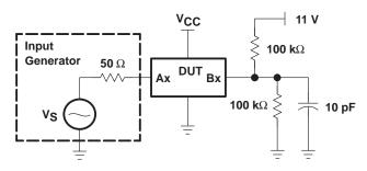
Figure 1. Device Test Setup
