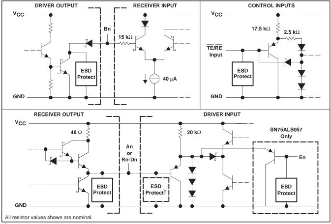
† Additional ESD protection is on the SN75ALS057, which has separate receiver-output and driver-input pins.
