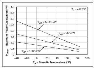
Results shown are with no air flow and PCB size of 3 in  $\times$  3 in (76.2 mm  $\times$  76.2 mm).
