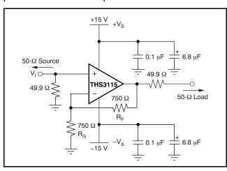
Figure 39. Wideband, Noninverting Gain Configuration
