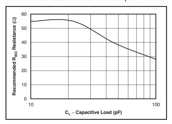
Figure 43. Recommended R<sub>ISO</sub> vs Capacitive
