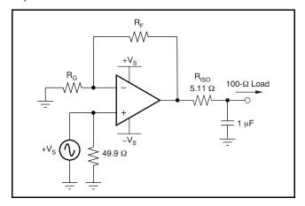
Figure 44. Resistor to Isolate Capacitive Load
