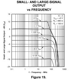
**SMALL- AND LARGE-SIGNAL** OUTPUT vs FREQUENCY
