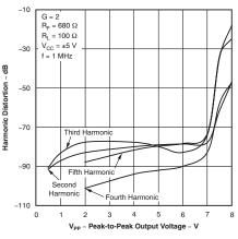
HARMONIC DISTORTION vs PEAK-TO-PEAK OUTPUT **VOLTAGE**
