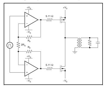
Figure 49. PowerFET Drive Circuit
