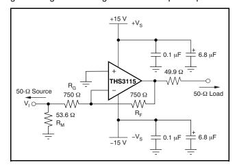
Figure 40. Wideband, Inverting Gain Configuration
