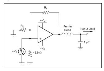
Figure 45. Ferrite Bead to Isolate Capacitive Load
