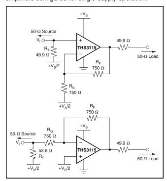
Figure 41. DC-Coupled, Single-Supply Operation
