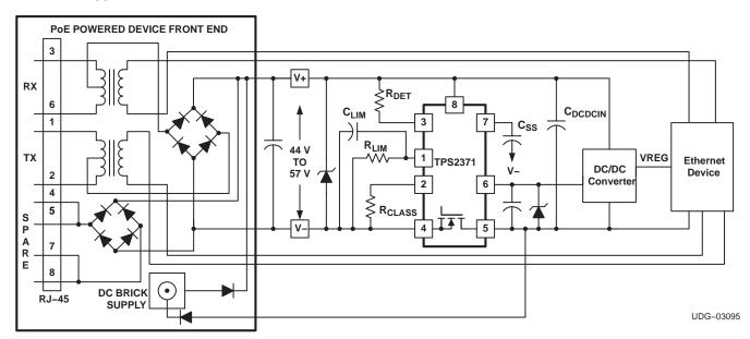
Figure 2. For Applications  $V_{IN}$  < 40 V.
