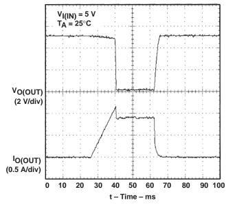
Figure 6. TPS2042, Short-Circuit Current, Device Enabled into Short
