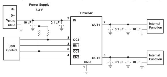
Figure 32. High-Power Bus-Powered Function
