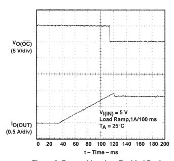
Figure 9. Ramped Load on Enabled Device
