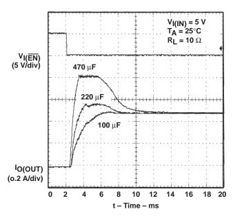
Figure 8. Inrush Current with 100-μF, 220-μF and 470-μF Load Capacitance
