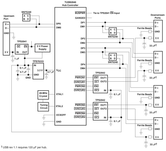
Figure 33. Hybrid Self/Bus-Powered Hub Implementation
