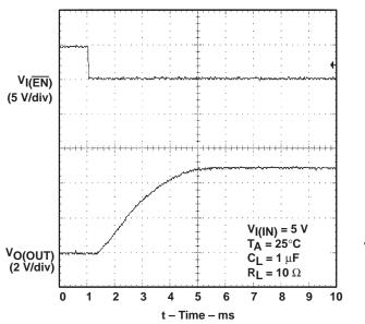
VI(EN) (5 V/div)  $V_{I(IN)} = 5 V$  $T_A = 25^{\circ}C$ VO(OUT)  $C_L = 1 \mu F$ (2 V/div)  $R_L = 10 \Omega$ 2 4 6 8 10 12 18 20 t - Time - ms
