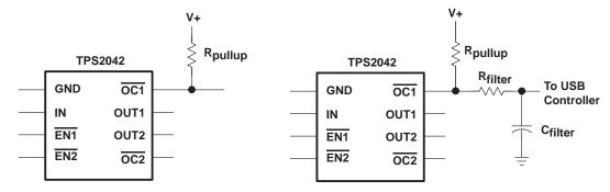
Figure 30. Typical Circuit for OC Pin and RC Filter for Damping Inrush OC Responses
