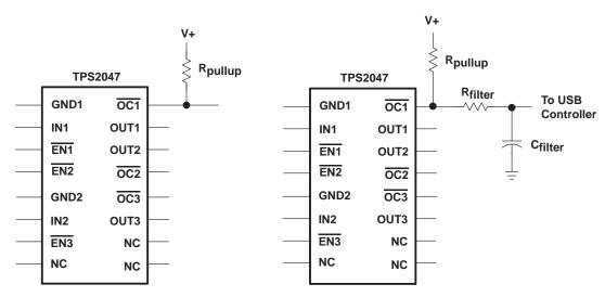
Figure 30. Typical Circuit for OC Pin and RC Filter for Damping Inrush OC Responses
