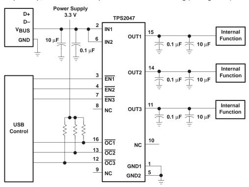
Figure 31. High-Power Bus-Powered Function
