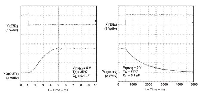
Figure 2. Turnon Delay and Rise Time with 0.1- $\mu$ F Load
