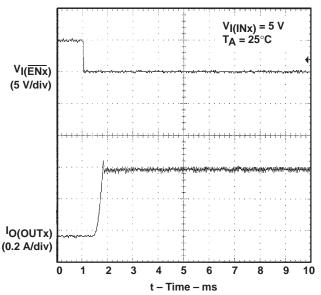
Figure 6. TPS2047, Short-Circuit Current,
