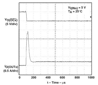
Figure 10. 4- $\Omega$  Load Connected to Enabled Device
