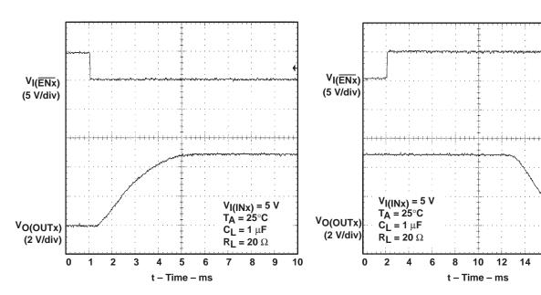
Figure 4. Turnon Delay and Rise Time with 1-µF Load
