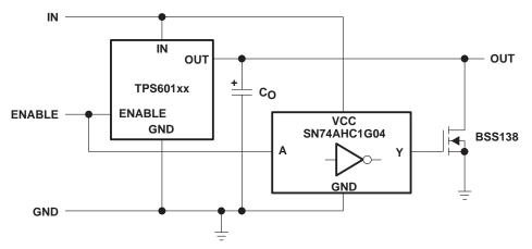
Figure 31. Block Diagram of the Regulated Discharge of the Output Capacitor
