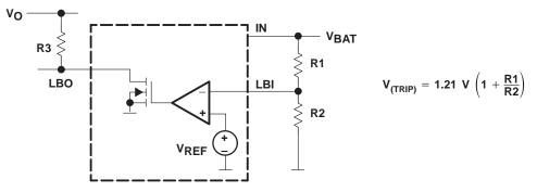
Figure 1. Programming of the Low-Battery Comparator Trip Voltage
