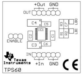
Figure 28. Component Placement
