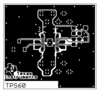
Figure 27. Recommended PCB Layout for TPS6012X
