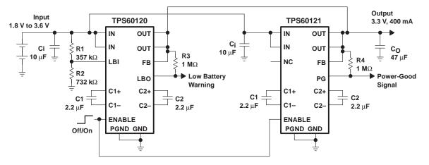
Figure 29. Paralleling of Two TPS6012x Charge Pumps
