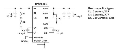
Figure 5. Circuit Used For Typical Characteristics Measurements
