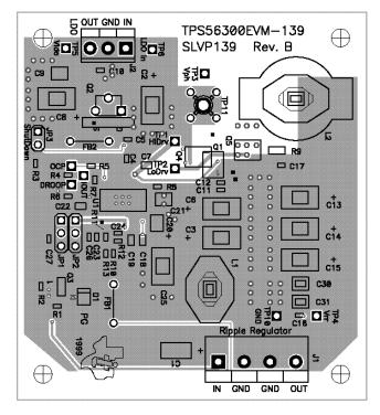
Figure 31. Bottom Layer (Top View)
