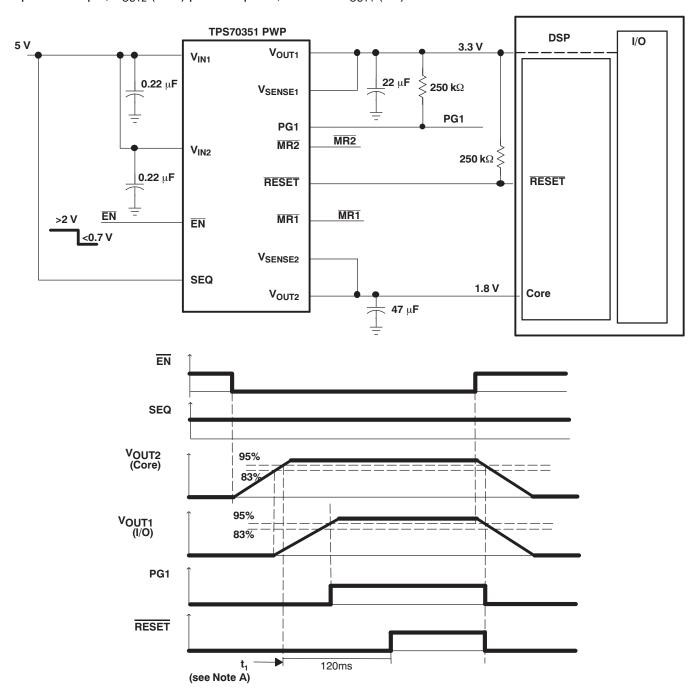
NOTE A:  $t_1$ : Time at which both  $V_{OUT1}$  and  $V_{OUT2}$  are greater than the PG thresholds and  $\overline{MR1}$  is logic high.
