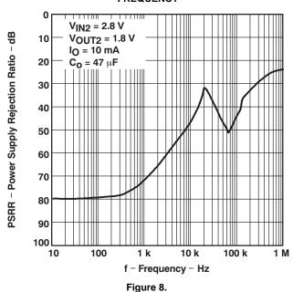
**TPS70351 POWER-SUPPLY REJECTION RATIO** vs **FREQUENCY**
