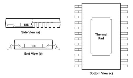
Figure 33. Views of Thermally-Enhanced PWP Package
