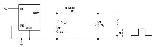
Figure 28. Test Circuit for Typical Regions of Stability
