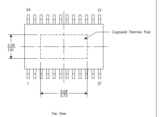
NOTE: A. All linear dimensions are in millimeters
