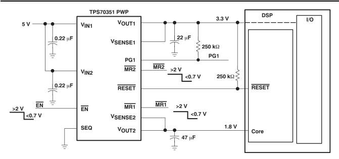
The TPS703xx family of voltage regulators offers very low dropout voltage and dual outputs with power up sequence control, designed primarily for DSP applications. These devices have low noise output performance without using any added filter bypass capacitors, and are designed to have a fast transient response and be stable with 47  $\mu$ F low ESR capacitors.
