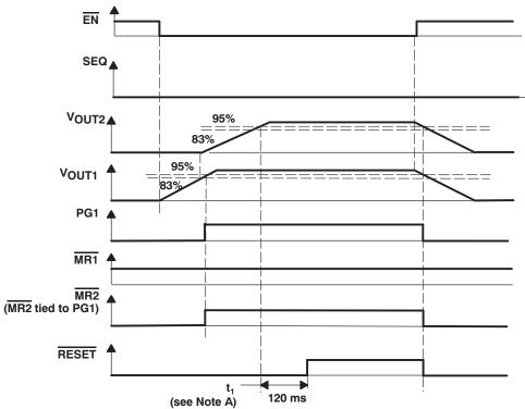
NOTE A:  $t_1$ : Time at which both  $V_{OUT1}$  and  $V_{OUT2}$  are greater than the PG thresholds and  $\overline{MR1}$  is logic high.
