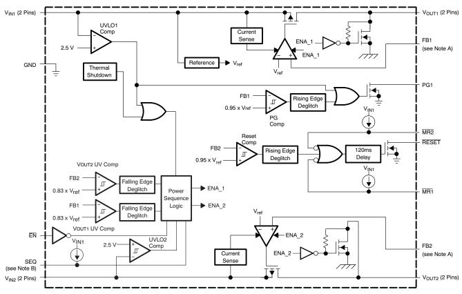
A. For most applications,  $V_{SENSE1}$  and  $V_{SENSE2}$  should be externally connected to  $V_{OUT1}$  and  $V_{OUT2}$ , respectively, as close as possible to the device. For other implementations, refer to SENSE terminal connection discussion in the *Application Information* section.
