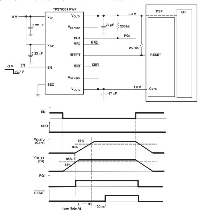
NOTE A:  $t_1$ : Time at which both  $V_{OUT1}$  and  $V_{OUT2}$  are greater than the PG thresholds and  $\overline{MR1}$  is logic high.
