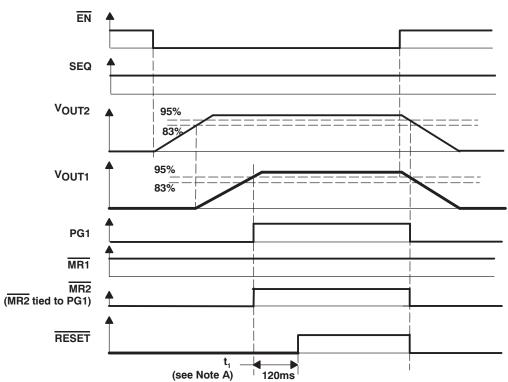
NOTE A:  $t_1$ : Time at which both  $V_{OUT1}$  and  $V_{OUT2}$  are greater than the PG thresholds and  $\overline{MR1}$  is logic high.
