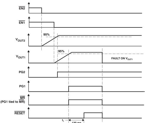
NOTES: A.  $t_1$ : Time at which  $V_{IN}$  is greater than  $V_{UVLO}$  and  $\overline{MR}$  is logic high. B. The timing diagram is not drawn to scale.
