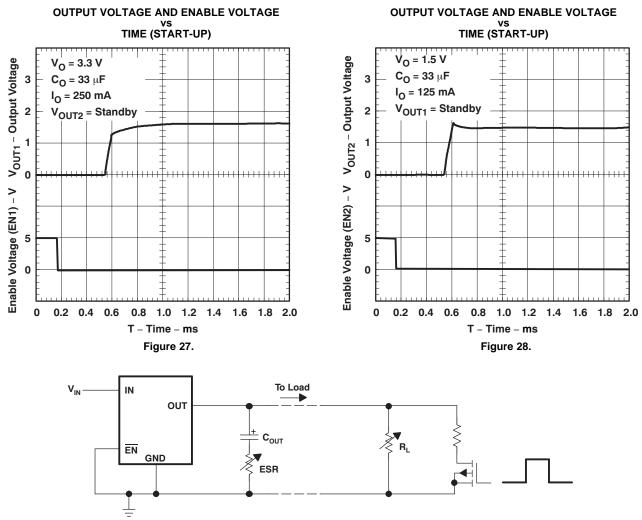
Figure 29. Test Circuit for Typical Regions of Stability
