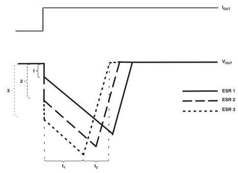
Figure 39. Correlation of Different ESRs and Their Influence on the Regulation of  $V_0$  at a Load Step from Low-to-High Output Current
