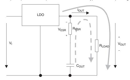
Figure 38. LDO Output Stage with Parasitic Resistances ESR
