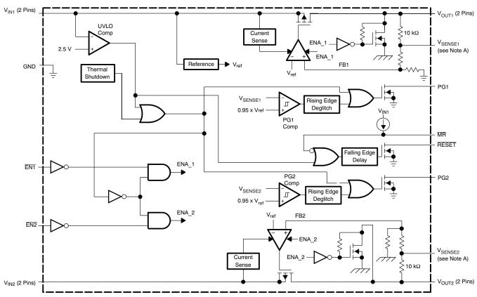
A. For most applications, V<sub>SENSE1</sub> and V<sub>SENSE2</sub> should be externally connected to V<sub>OUT1</sub> and V<sub>OUT2</sub>, respectively, as close as possible to the device. For other implementations, refer to SENSE terminal connection discussion in the *Application Information* section.
