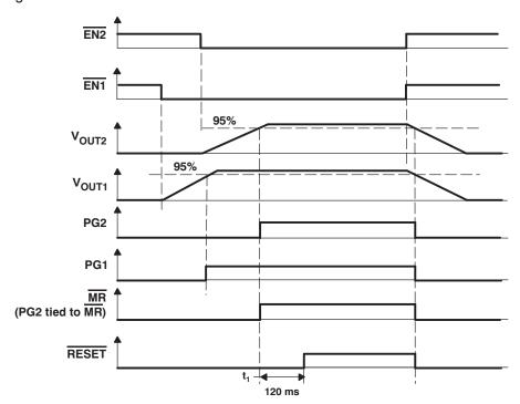
NOTES: A.  $t_1$ : Time at which  $V_{IN}$  is greater than  $V_{UVLO}$  and  $\overline{MR}$  is logic high. B. The timing diagram is not drawn to scale.
