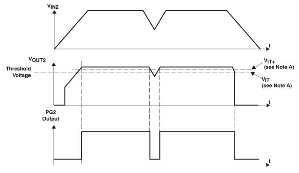
NOTE A:  $V_{IT_{-}}$  trip voltage is typically 5% lower than the output voltage (95% $V_{0}$ ).  $V_{IT_{-}}$  to  $V_{IT_{+}}$  is the hysteresis voltage.
