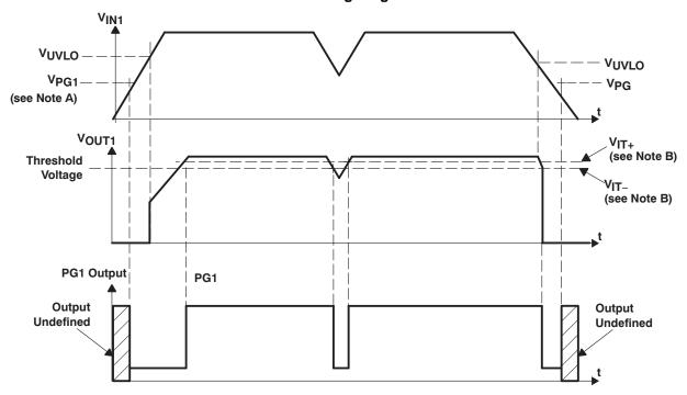
NOTES A:  $V_{PG1}$  is the minimum input voltage for a valid PG. The symbol  $V_{PG1}$  is not currently listed within EIA or JEDEC standards for semiconductor symbology.
