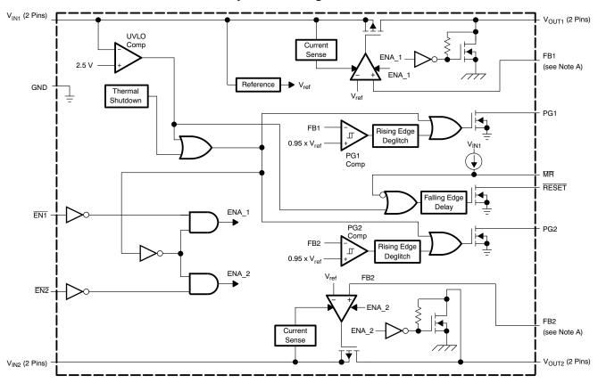
A. For most applications, FB1 and FB2 should be externally connected to resistor dividers as close as possible to the device. For other implementations, refer to FB terminals connection discussion in the *Application Information* section
