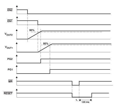
NOTES: A.  $t_1$ : Time at which  $V_{IN}$  is greater than  $V_{UVLO}$  and  $\overline{MR}$  is logic high. B. The timing diagram is not drawn to scale.
