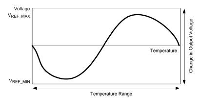
Figure 25. Illustrative V<sub>REF</sub> vs Temperature Profile
