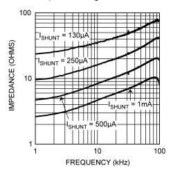
Figure 22. Reverse Dynamic Impedance vs IOUT
