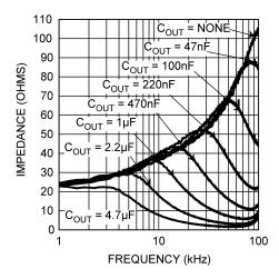
Figure 23. Reverse Dynamic Impedance vs Cout
