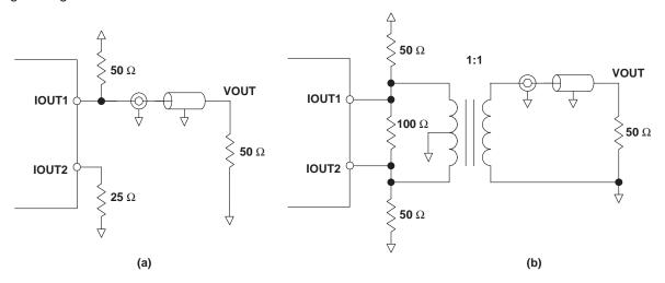
Figure 28. Driving a Doubly Terminated 50  $\Omega$  Cable
