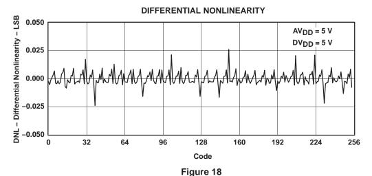
$^\dagger$  AV<sub>DD</sub> and DV<sub>DD</sub> specified for each chart seperately, IOUTFS = 20 mA, single-ended output IOUT1, 50  $\Omega$  doubly terminated load, T<sub>A</sub> = 25°C (unless otherwise noted.)
