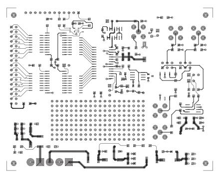
Figure 30. Board Layout, Layer 1
