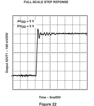
$^\dagger$  AV<sub>DD</sub> and DV<sub>DD</sub> specified for each chart seperately, IOUT<sub>FS</sub> = 20 mA, single-ended output IOUT1, 50  $\Omega$  doubly terminated load, T<sub>A</sub> = 25°C (unless otherwise noted.)
