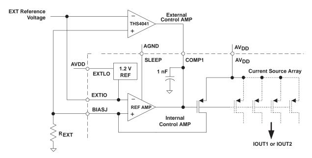
Figure 25. Bypassing the Internal Reference and Control Amplifier
