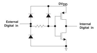
Figure 24. Digital Equivalent Input
