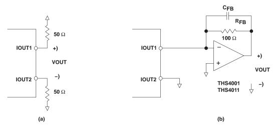
Figure 27. Differential and Single-Ended Output Configuration
