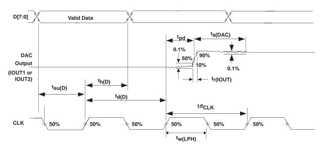
Figure 23. Timing Diagram
