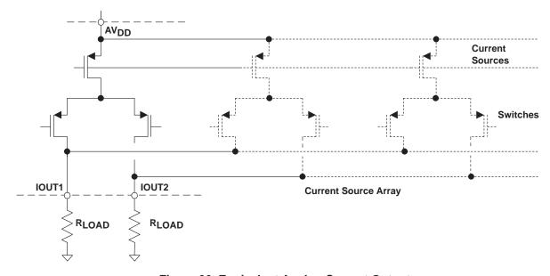
Figure 26. Equivalent Analog Current Output
