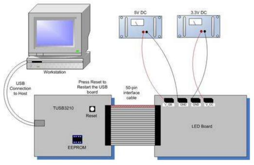
Quick Connection Diagram for LED Driver Boards
