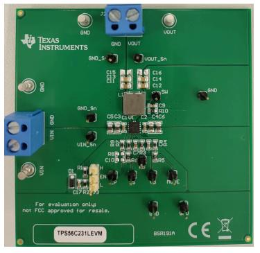
Figure 6-1. Top View of TPS56C231LEVM
