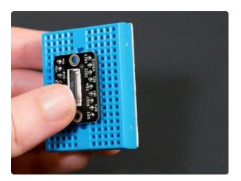
Then, insert the EYESPI cable into the open FPC connector by sliding the cable into the connector. You want to see the blue stripe facing up towards you. This inserts the cable pins into the FPC connector.
