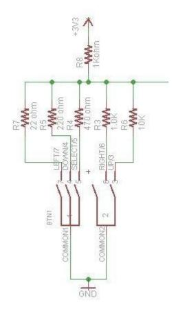
In the code example below, the CheckJoystick() function reads the analog pin and compares the result with 5 different ranges to determine which (if any) direction the stick has been moved. If you upload this to your Arduino and open the Serial Monitor, you will see the current joystick state printed to the screen.
