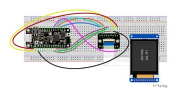
breakout Vin to Feather 3.3V (red wire) breakout Lite to Feather 3.3V (yellow wire) breakout Gnd to Feather GND (black wire) breakout SCK to Feather SCK (grey wire) breakout MISO to Feather MI (green wire) breakout MOSI to Feather MO (purple wire)
