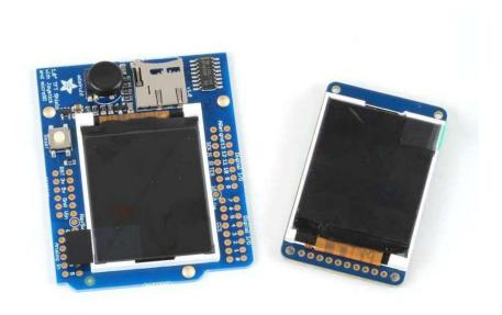
The 1.8" display has 128x160 color pixels. Unlike the low cost "Nokia 6110" and similar LCD displays, which are CSTN type and thus have poor color and slow refresh, this display is a true TFT! The TFT driver (ST7735R) can display full 18-bit color (262,144 shades!). And the LCD will always come with the same driver chip so there's no worries that your code will not work from one to the other.
