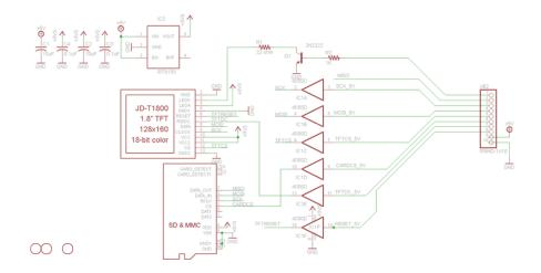
For the level shifter we use the CD74HC4050 which has a typical propagation delay of  $^{\sim}10$ ns
