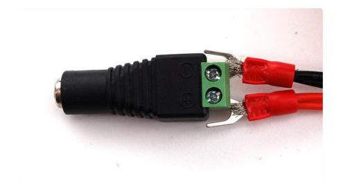
You may receive power cables with different endings, e.g. round instead of spade ends, or maybe with another Molex connector. Just strip the cables and wire directly to the power plug
