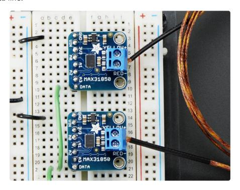
The MAX31850K data format is very similar to that of the well known 1-Wire DS18B20 temp sensor but it is not drop in compatible without code changes to check for the new '1 Wire family' type. We have adapted the classic Arduino <a href="OneWire">OneWire</a> () and <a href="DallasTe">DallasTe</a> <a href="Max31850">mp</a> () libraries to be MAX31850 compatible, so please click on those links to grab our libraries.
