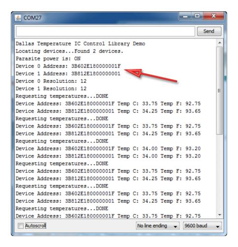
Note that this address is not connected to the ADDR pins on the breakout! those are different address pins. You cannot change the 64-bit address, its permanently burned into the chip!
