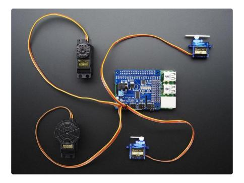
The Raspberry Pi is a wonderful little computer, but one thing it isn't very good at is controlling DC Servo Motors - these motors need very specific and repetitive timing pulses to set the position. Instead of asking the Pi Linux kernel to send these signals, pop on our handy HAT or Bonnet.
