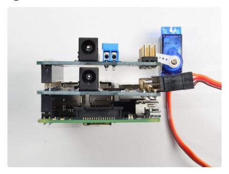
Even though HATs are not intended to be stacked, you can stack up to 62 HATs and not have an address collision, for up to 992 PWM outputs! You'll still need to provide power and write code for all those outputs but they can all share the same SDA/SCL pins no problem.
