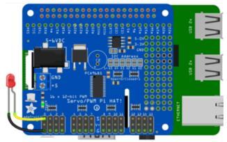
Connect LED cathode / shorter leg to HAT or Bonnet channel GND / ground.
