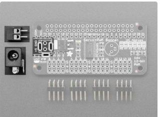
The power input section of the HAT and Bonnet are both on the left hand side.
