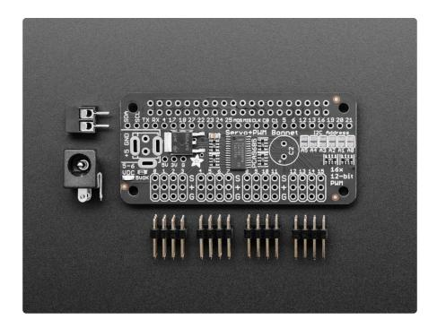
The Adafruit 16-Channel 12-bit PWM/Servo HAT or Bonnet will drive up to 16 servos or PWM outputs over I2C with only 2 pins. The on-board PWM controller will drive all 16 channels simultaneously with no additional Raspberry Pi processing overhead. What's more, you can stack up to 62 of them to control up to 992 servos - all with the same 2 pins!
