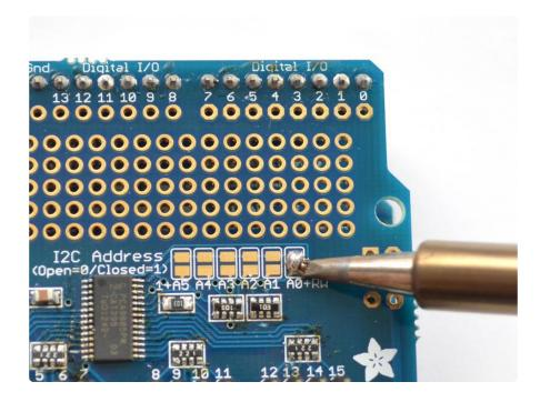
Board 0: Address = 0x40 Offset = binary 00000 (no jumpers required)
