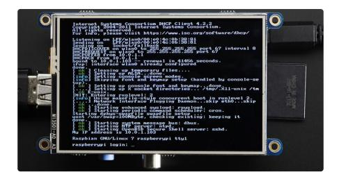
One fun thing you can do with the display is have it as your main console instead of the HDMI/TV output. Even though it is small, with a good font you can get  $20 \times 40$  of text. For more details, check out https://github.com/notro/fbtft/wiki/Boot-console ()
