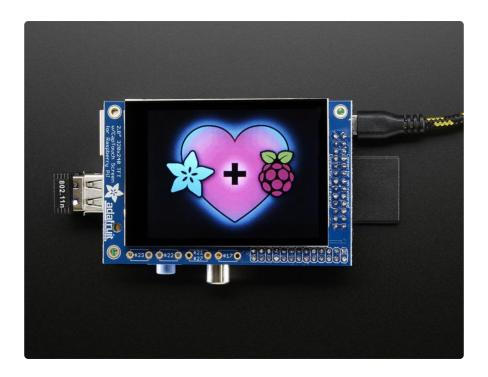
Uses the hardware I2C Pins (SDA & SCL), SPI pins (SCK, MOSI, MISO, CE0) as well as GPIO #25 and #24. All other GPIO are unused. Since we had a tiny bit of space, there's 4 spots for optional slim tactile switches wired to four GPIOs, that you can use if you want to make a basic user interface. For example, you can use one as a power on/off button. See below for the link to get the optional tact switches, they're not included.
