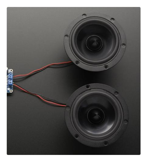
Don't forget to gently yank on each wire after clamping it into the terminal block, it should be a solid connection, not possible to yank out of place. Loose wires will be a problem!
