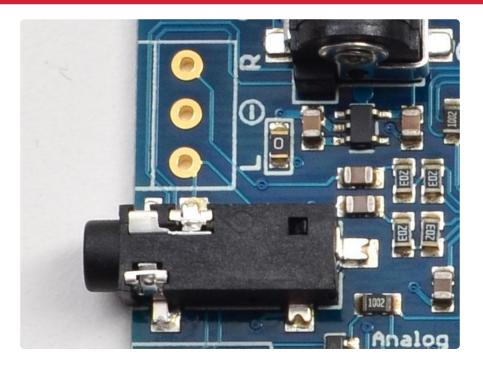
The headphone jack is a classic 3.5mm as seen in just about every audio device. You can connect this directly to any audio output. The terminal blocks are for if you have some direct-wiring project and you want a more permanent connection. You'll have to solder in the terminal blocks if you want to use that technique, see the Assembly page
