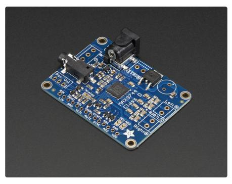
Pump up the volume with this 20W stereo amplifier! This slim little board has a class D amplifier onboard that can drive 2 channels of 4-8 ohm impedance speakers at 20W each. Power it with 5-12VDC using the onboard DC power jack and plug stereo line level into the 3.5mm stereo headphone jack and jam out with ease. Since it's class D, its completely cool-running, no heat sinks are required and it's extremely efficient - up to 93% efficiency makes it great for portable or battery powered rigs.
