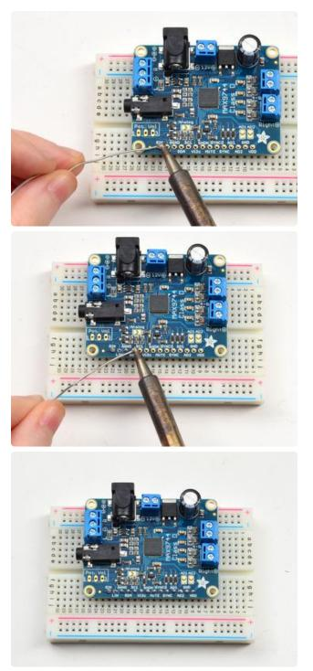
Solder in all of the header pins to the breakout board.
