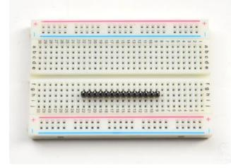
Break off a piece of 0.1" male header, 14 pins long and stick it long pins down into the solderless breadboard
