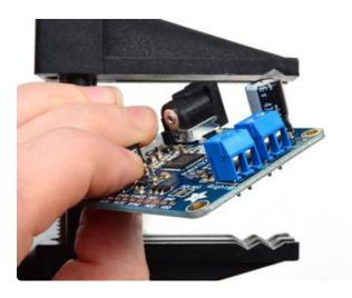
Place two of the 2-pin blue terminal blocks so that the holes point outward
