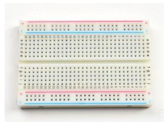
The easiest way to attach headers to the breakout board is to take advantage of a solderless breadboard you may have.
