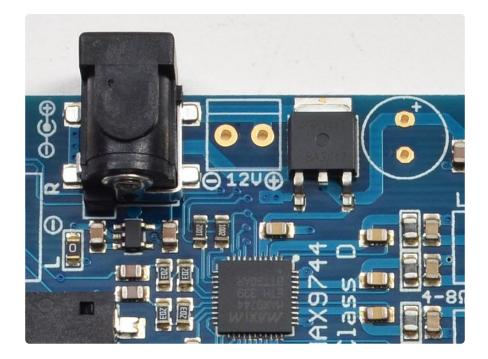
There's two ways to get power into this board, either by the 2.1mm DC jack (on the left) or the 3.5mm terminal block breakout (in the middle). Both are connected up together so use whichever you like.
