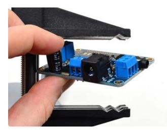
Place the 2-pin and 3-pin terminal blocks so the holes point out
