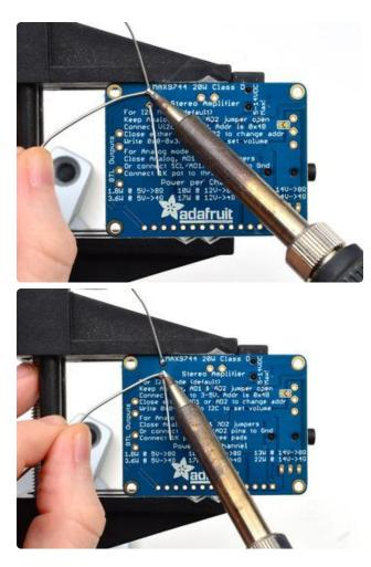
pins at the same time with the edge of the soldering iron and dipping a little solder in.
