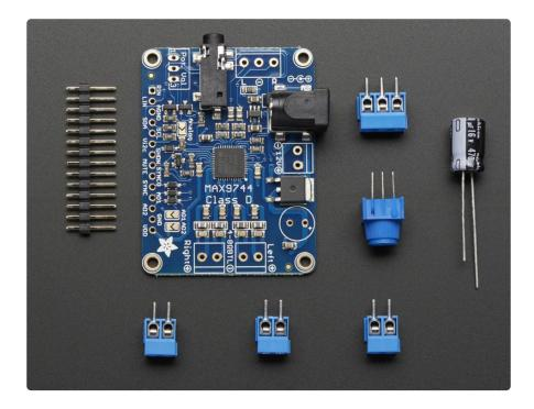
Each order comes with one MAX9744 breakout board with all surface-mount parts fully assembled and tested. We also include 3 x 2pin and 1 x 3pin terminal blocks, a 470 $\mu$ F power filter capacitor and 1K $\Omega$  trim pot. To use this board, a little soldering is
