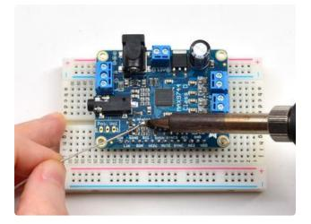
Finally, solder closed the Analog jumper on the left side.
