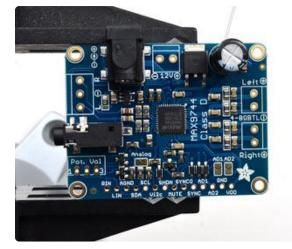
Place the capacitor against the PCB and bend the two leads out so that it sits flat.
