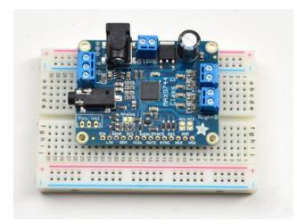
This will keep it in place when you put the audio amplifier on top! Put the breakout board onto the short header pins so they stick out thru the breakout pads
