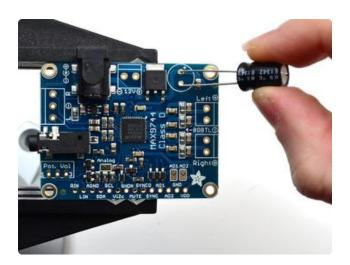
Capacitors are polarized, they have to be placed in the right way! The longer lead goes into the pad marked +
