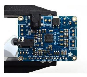
Begin by placing the amplifier board in a vise so you can easily work on it. Heat up your soldering iron to 650-700 degrees F and get some solder and hand tools ready!
