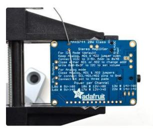
Flip over the board so you can solder the two pads
