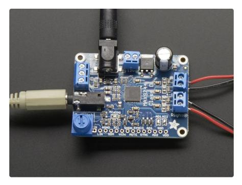
Once you have that working, you can solder wires to the Pot Vol pads, so you can place the volume adjustment pot elsewhere (say mounted to the outside of a box)
